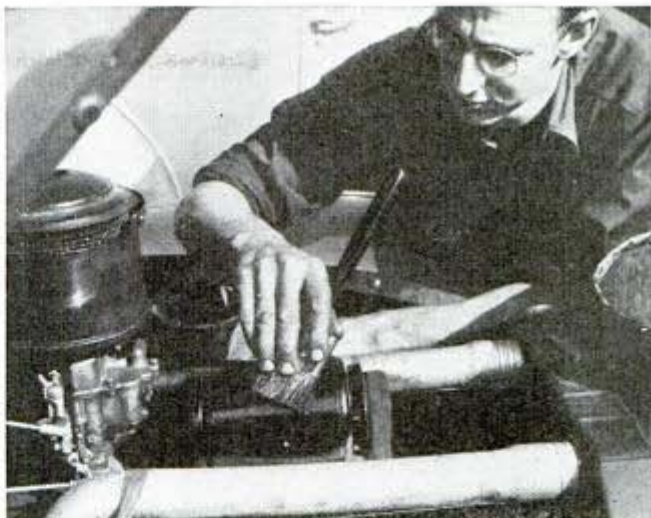
Keep your engine clean, using a solvent occasionally to brush the dirt away. The engine that is free of dust and oily grime will run perceptibly cooler in summer weather
